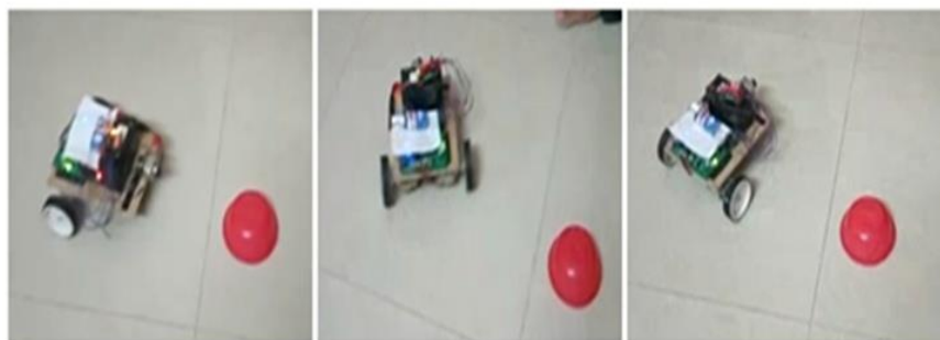
Figure 7: The final robot prototype and its movement by avoiding the obstacle(red in colour)
